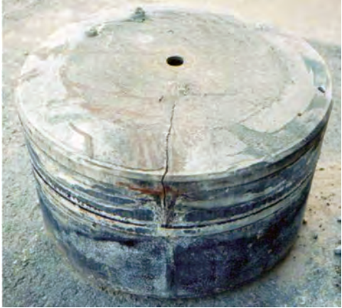
Severely cracked 6500 dolly should be replaced.
