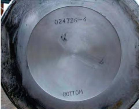
View showing underside of 4500 dolly after 150 hrs of work. No signs of cracking. OK.
