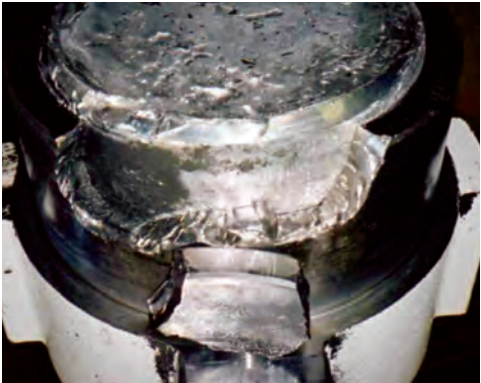
If dolly is not replaced when it has been overworked, the anvil body can break due to expansion of dolly material.
