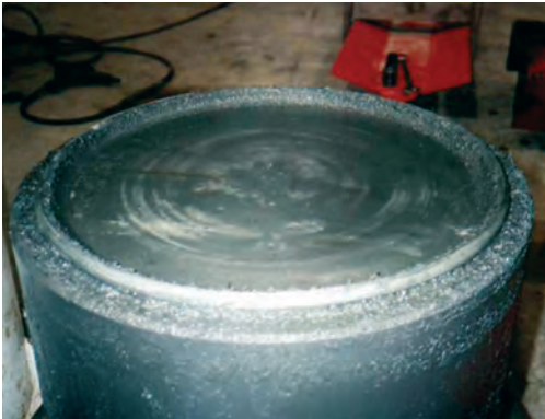
Overworked 6500 dolly stuck in anvil body, must be replaced or it can cause the anvil body to break.
