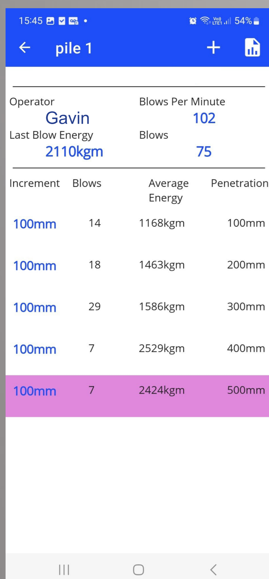
DAWSON PILE LOGGER SCREEN
