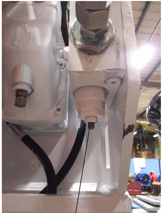
Flow Compensator 8.5mm (default setting)
