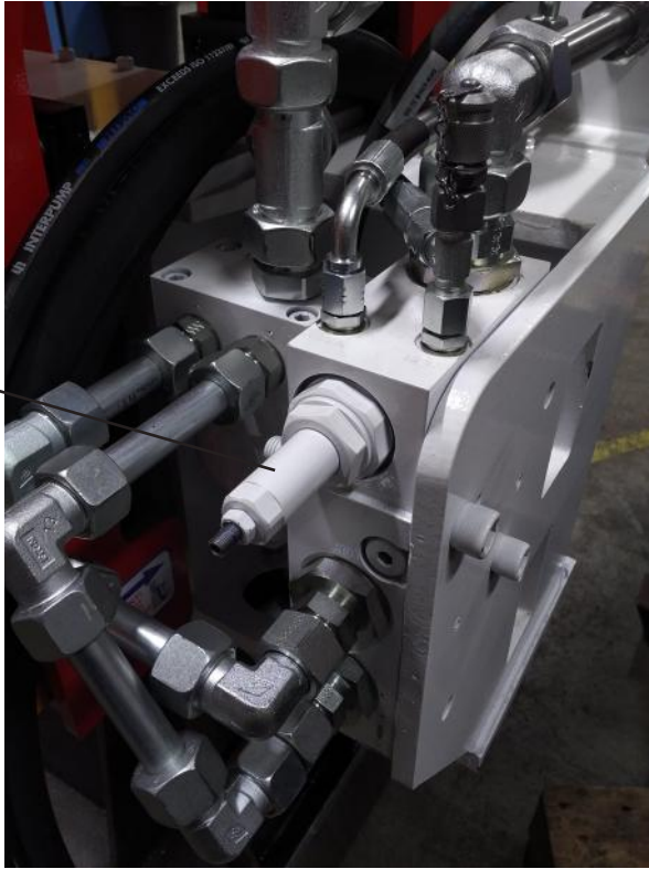
Sequence valve 11.5mm (default setting)
