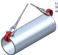
Lifting Angle Range: 30-45° (measured from vertical). Sling Legs must be of equal length. Angles greater than 45° will result in over-loading the equipment.
