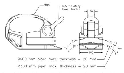
Lifting pipes using Dawson's Pipe Handling Shoes increases the range of steel pipe that can be handled, and also the load capacity:
