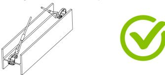
This is the correct method for lifting H-section beams with two pairs of 900 shoes. A short chain should also be connected between the pairs of shoes to prevent them from spreading as shown in the diagram below.
